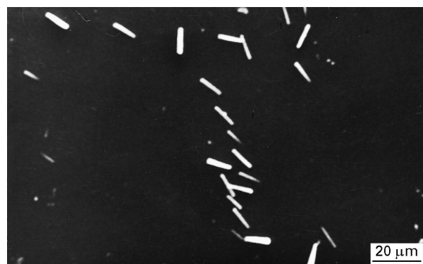
Figure 3 Micrograph of a \text{CN}_x layer surface containing small grains.
